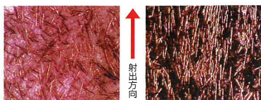
ガラス繊維: 30wt% Glass fiber: 30wt% パナテトラ: 10wt% "Pana-Tetra": 10wt%
